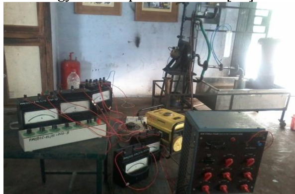
Figure – 3 Experimental set up for Power quality analysis of Inductive load with biomass gasifier
