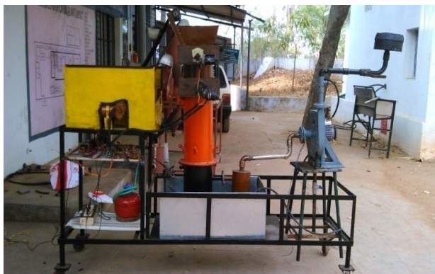
Figure 2: Fabricated 2kW Biomass Gasifier
