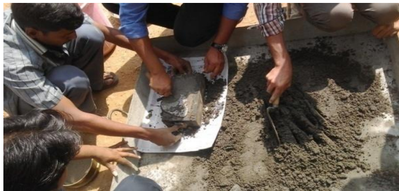
Figure 1: Casting the Steel Slag Brick
