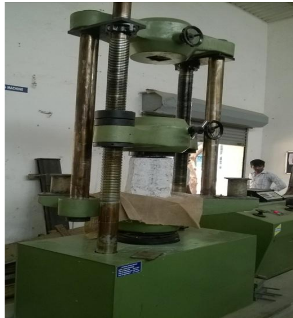
Figure 4: Test setup of steel slag brick prism
