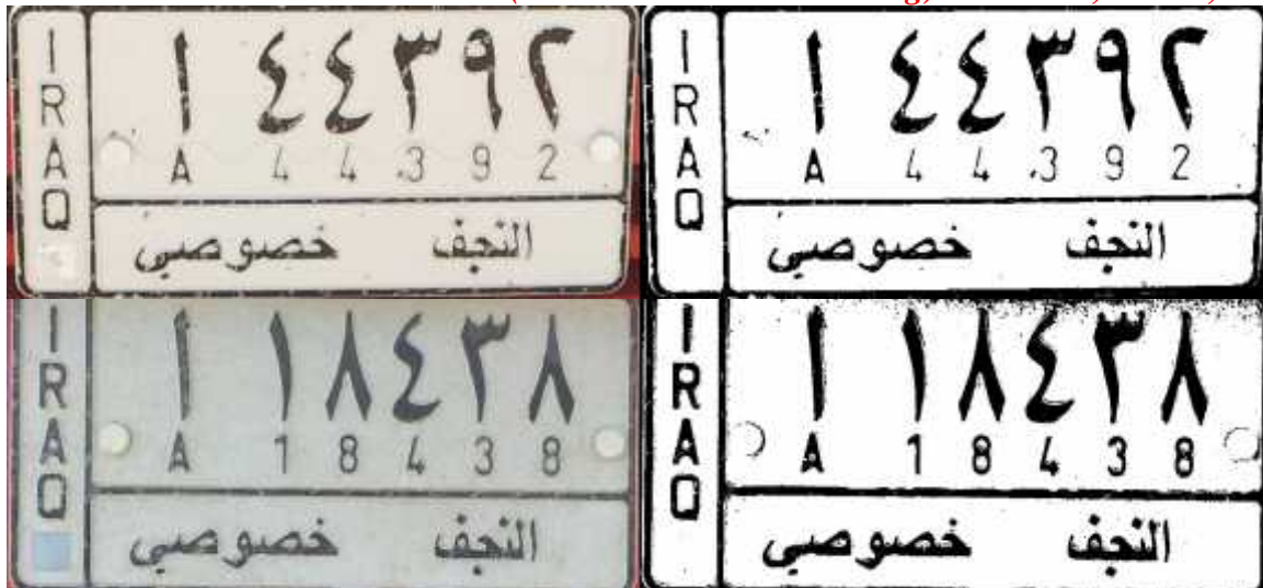
Figure 2. License plate image after localization and pre-processing
