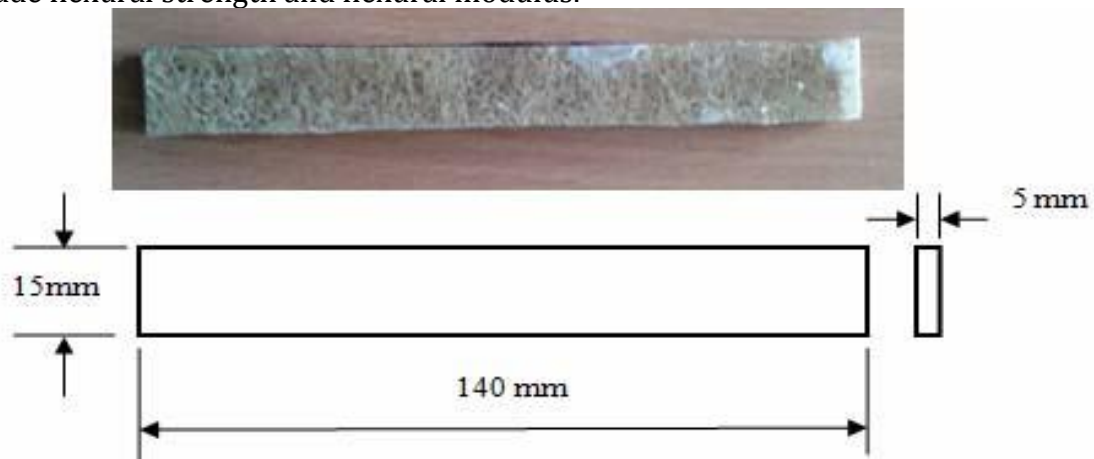
Figure 5: Flexural test specimen as per ASTM D790.
