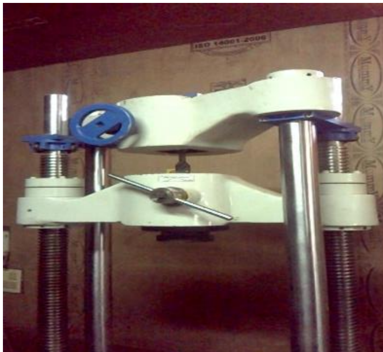
Figure 4: UTM 1000KN make FIE with tensile specimen at the time of testing
