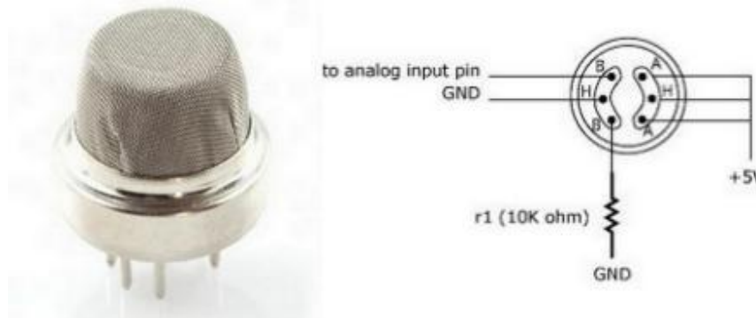
Figure (5): Pin Configuration of Gas Sensor
