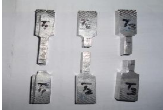
Figure 4 - Tensile tested specimen (T 1 -3%, T 2 -6%, T 3 -12%)
