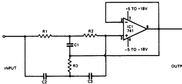
Figure (6): Notch filter
