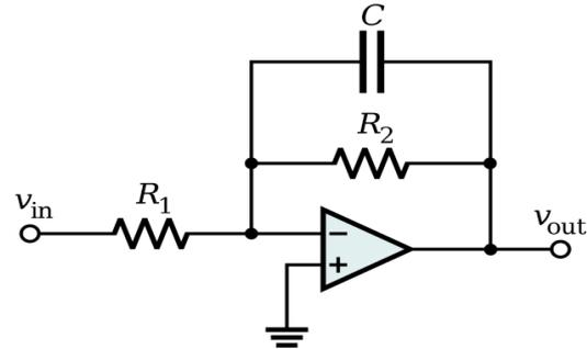
Figure (7): Low pass filter/Amplifier
