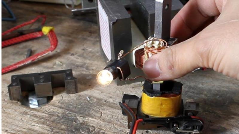
Figure 1: Wireless Bulb by Electromagnetic Induction
