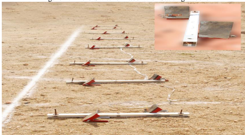
Figure 1: Micro Switches Fitted With Starting Blocks
