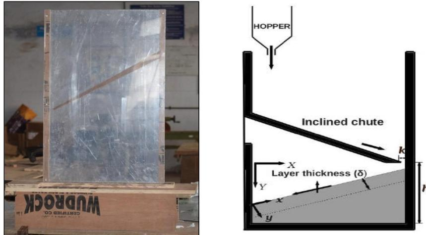
Figure 1: Experimental setup and schematical diagram of the Quasi 2 dimensional model
