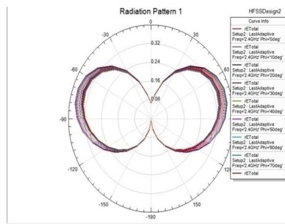
Figure 3(b): Radiation pattern of the antenna in light on state
