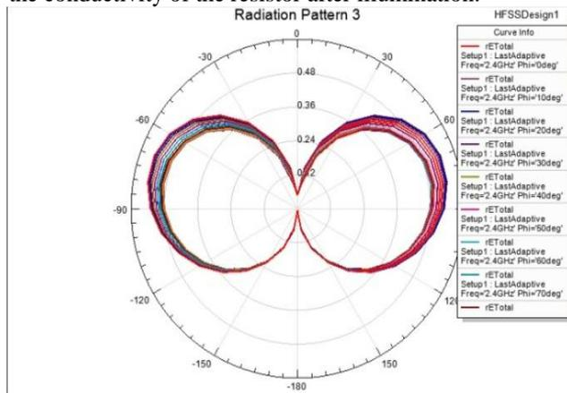
Figure 3(a): Radiation pattern of the antenna for light off state
