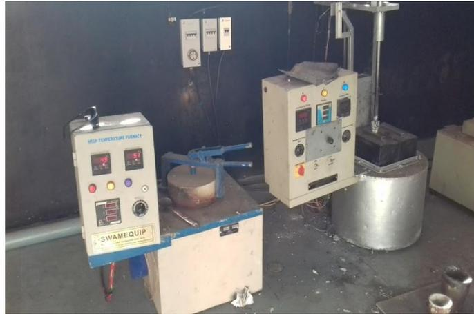
Figure 1: Stir Casting Set Up
