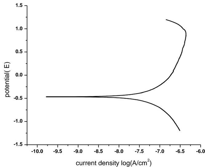
Figure 5: Tafel plot of corrosion behaviour of 1.5wt% Ag-HAP
