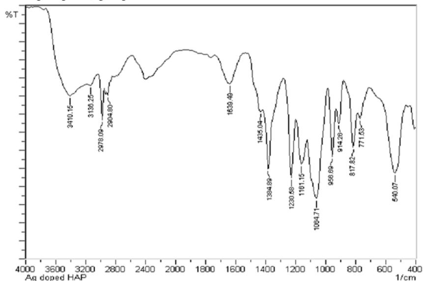
Figure 1: FTIR of pure Ag-HAP deposited on alumina
