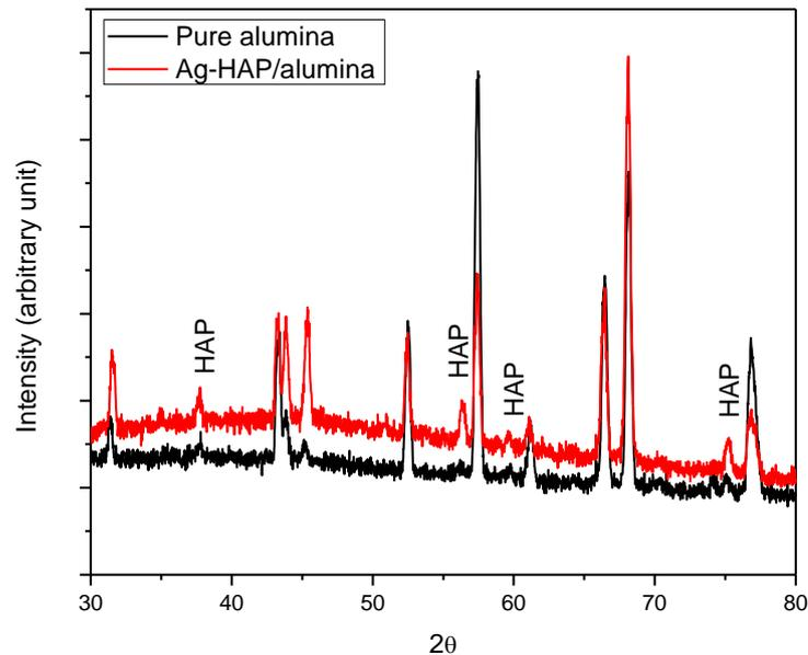
Figure 2: XRD of Ag-HAP coated on alumina
