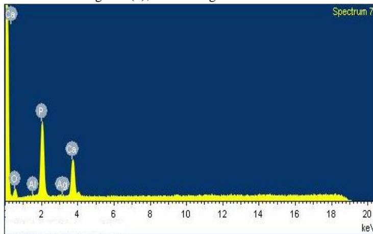
Figure 4: EDX of Ag-HAP/alumina showing the presence of Ag.
