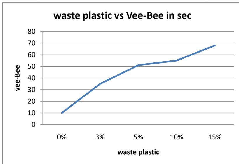
**Figure 5: Vee-Bee timing in seconds for different percentage of waste plastic**
