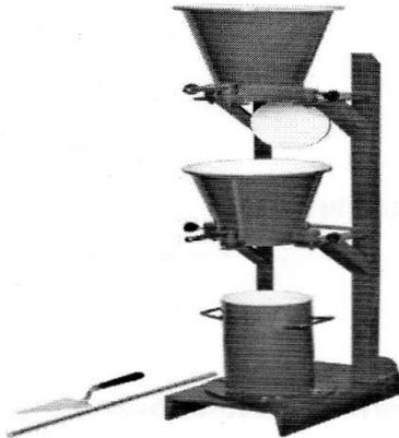
**Figure: Compacting factor apparatus**
