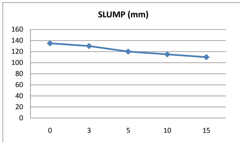
**Figure 1: Workability Graph (slump in mm)**
