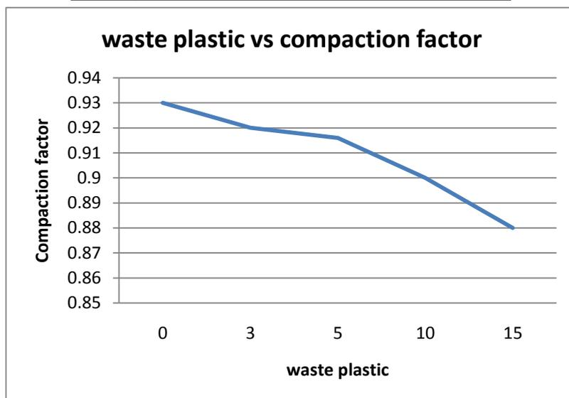
**Figure 3: Showing compaction factor values for different percentage of plastic**
