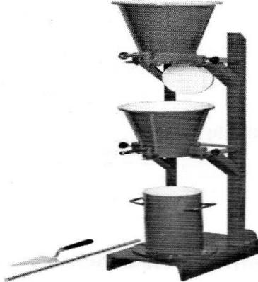
**Figure: Compacting factor apparatus**
